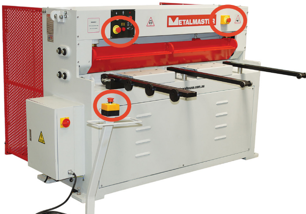
E: Emergency Stop
